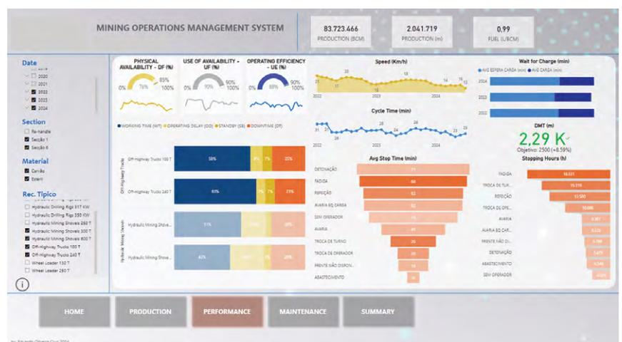
Figura 5 - Dashboard Mining Operations Management System ("Desempenho" - Dumpers).
